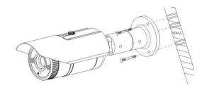
Step one: Measure the height of installation on wall and mark the holes positions. Step two: Drill the holes according to the measurement on wall. Step three: Put the expansion bolt in the drilled hole. Step four: Fix camera bracket hole by screws
